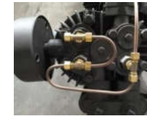
C: inlet unloader
